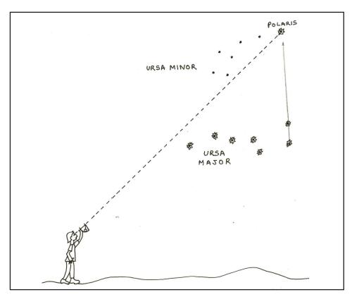
15. Measure the angle, it should be about 53°. That is the same as the latitude you are on! One very useful application for this information is to help you make or aligning a sundial. The pointer or Gnomon is most accurate when it is inclined at an angle equivalent to your latitude! See if you can find out why?
