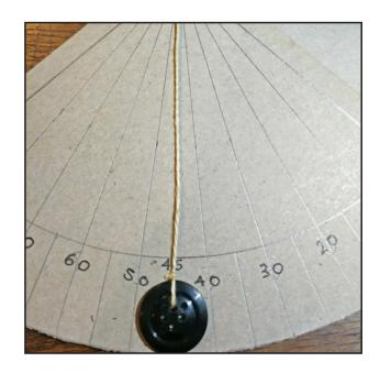
10. Next, carefully tape your backsight on, by the 90 degree line on the edge of the device. Next tape your foresight on the same edge as the backsight, by the origin, but on the back.
