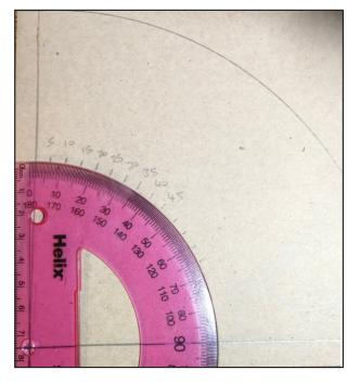
4. Before drawing the radial lines in, its probably better to draw a second arc. Measure 30mm from the existing arc.and draw a second one.
