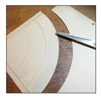
6. At the same time you can cut out a 'foresight' and a 'backsight'.These are what you use to align the device when taking a reading.The foresight is a rectangle of cardboard 10mm. by 20mm.The backsight is similar, 20mm by 30mm. with a hole punched through.Sometimes, cardboard dividers come pre punched, so you don't need a hole punch with them.
